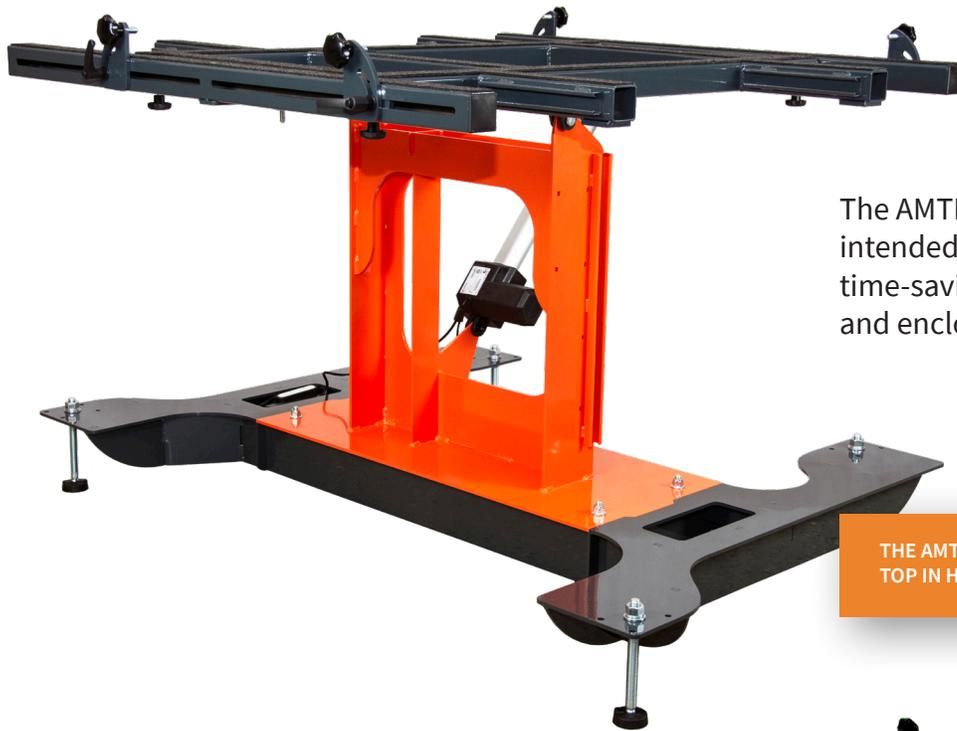
The AMTE-300 is a versatile assembly table intended for the ergonomic, effective, and time-saving assembly of electrical panels and enclosures.
